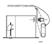
Attach the conduit fitting, lock nut, and safety chain bracket. Install a safety chain/cable (not supplied) that will support up to 16 pounds (7.3 kg).
